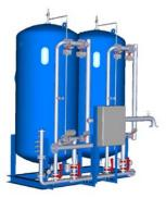
The resin beads in the regenerated state have a high concentration of sodium ions. These sodium ions have a relatively low electrical potential compared to that of calcium and magnesium, ions. This means ions with a greater potential or charge can easily replace them. When the inlet water flows through a cation resin bed, the calcium and magnesium ions bond to the resin beads, and the beads release sodium ions in exchange.
